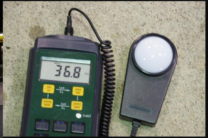
BEFORE 458w Metal Halide
